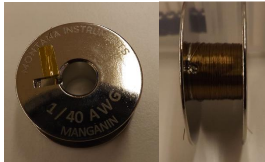
Figure 3: Manganin wire included with the accessory kit.
